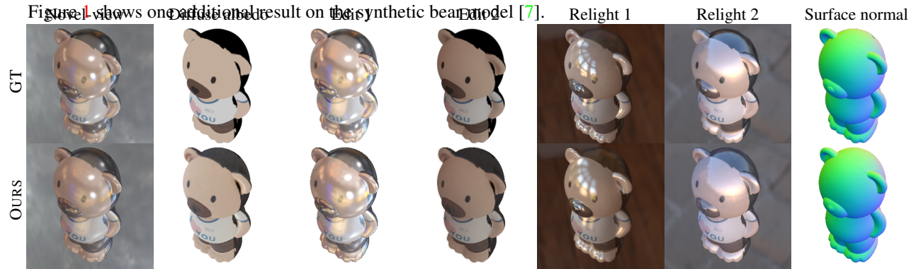
Figure 1: Results of our pipeline on synthetic data. For a novel test view, we compare our predicted image, estimated diffuse albedo, specular BRDF editing results and relighting results against the ground-truth rendered by Mitsuba [2].
